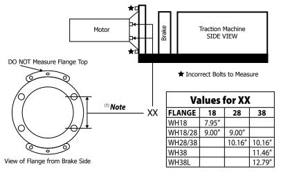
**Note:** Bolts to measure are hidden from normal view and are located behind the adapter.
